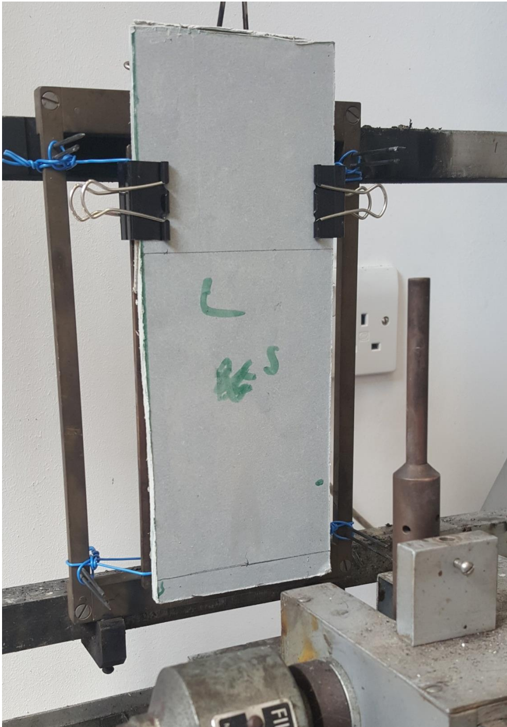
Photograph 4: Sample from Canute Garden cladding following single-flame source surface ignition test.
