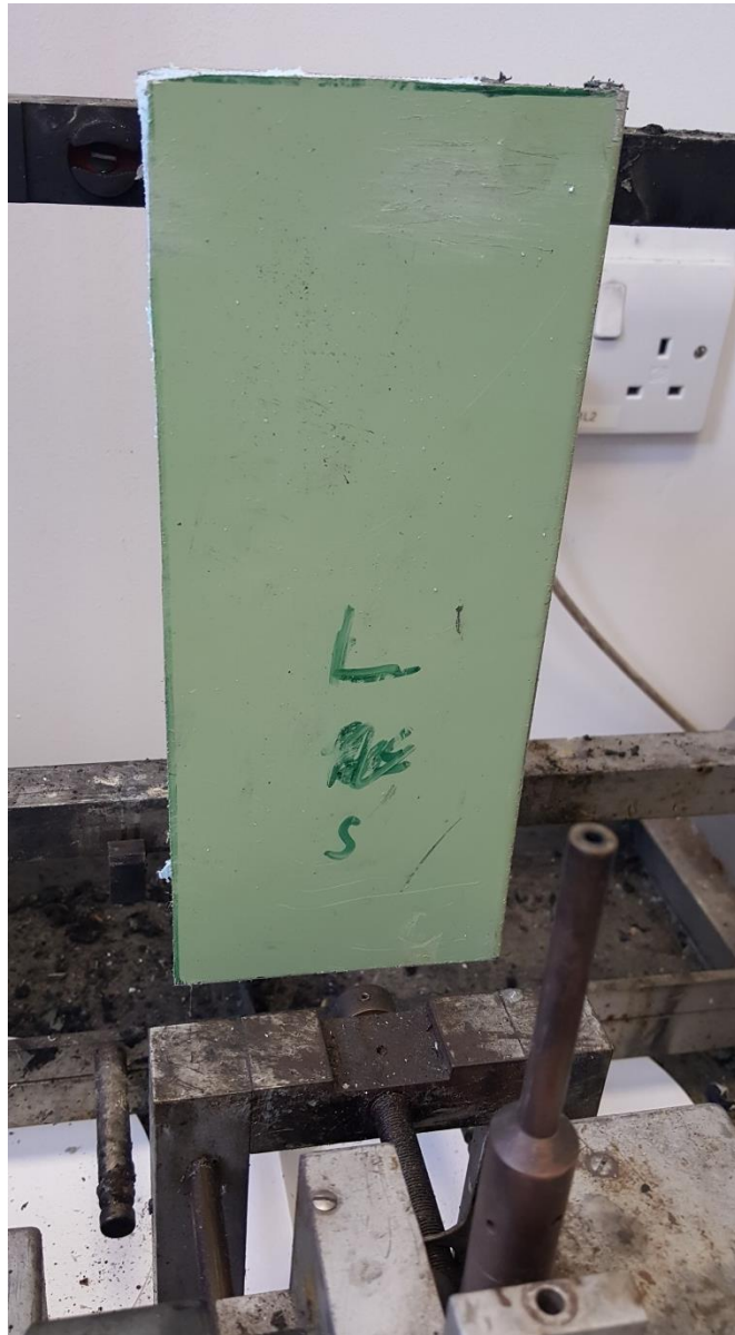
Photograph 6: Sample from Medina House cladding following single-flame source surface ignition test.
