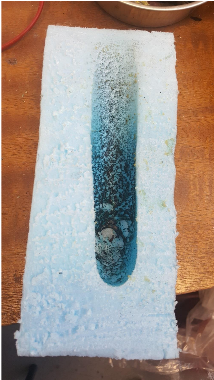
Photograph 8: Sample of the insulating foam from the Medina House cladding panels subjected to single-flame source surface ignition test.
